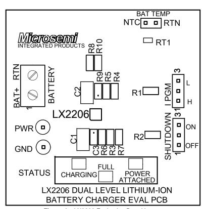
Figure 4 – LX2206 Evaluation Board Layout
